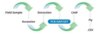
The PCR/SAP/EXT stage is where the laboratory partnered with Agena Bioscience® for a high-volume and low-cost alternative to RT-PCR testing—utilizing the MassARRAY® System that can process up to thousands of samples per day on a single machine for under \$10 per sample. Dr. Zanke elaborates on the process below:
